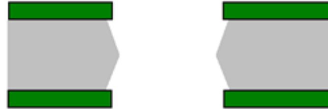
Double-side etching – „hour glass” cross-section
