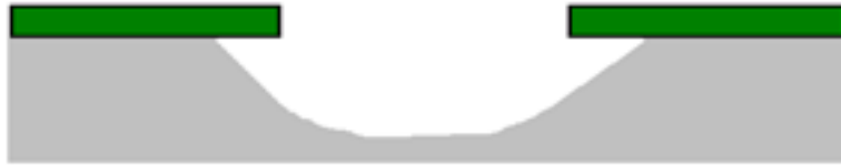
Single-side etching – high degree of undercutting
