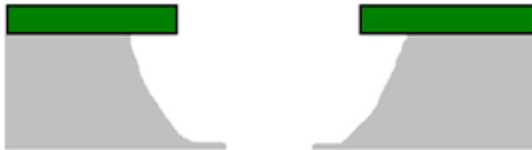
Single-side etching – formation of „knife-edge”
